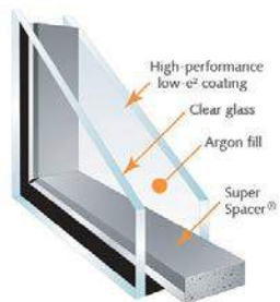
Illustration of a double glazed unit
